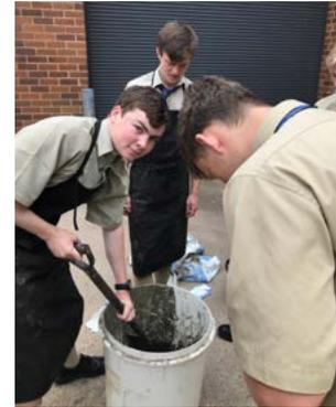
In Year 12 Engineering Studies, students as part of their unit on Civil Structures mixed and poured two concrete beams. One was reinforced with steel and the other without. After it has set for about a week they will test the relative strength of each beam
